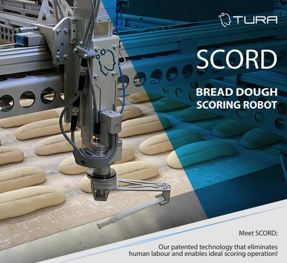
The 3D visioning system in SCORD scans every single dough on the production line with no mistake and creates unique 3D maps of each. It then calculates the ideal scoring path for each dough and transfers this information to its robotic subsystem. Our talented robot does the rest and creates perfect cuts on every dough. And it does not forget to clean its blade!
